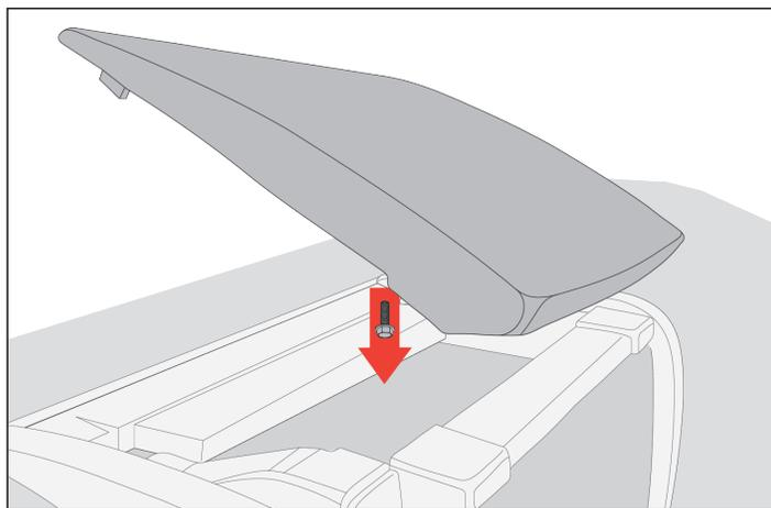
4. Install Multi-Mount Dash Storage by snapping front lip into dash, then pressing back tabs into place.
